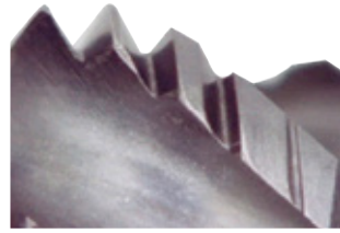
Enlarged Photo after tapped 250 holes by VUSP
